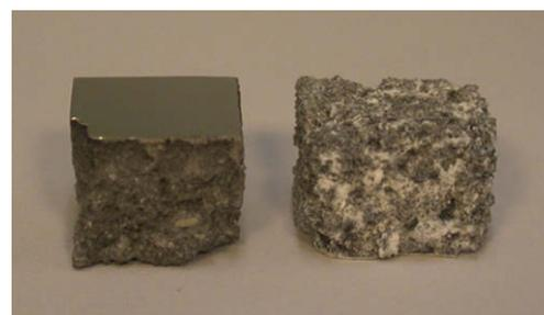
**Figure 3.** AZ91E sample with  $Al_3Mg_2$  coating on top (left) and AZ91E (right) after 48 h immersion test in 5% NaCl.
