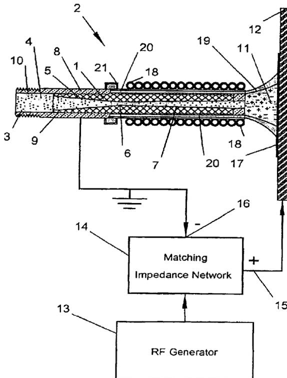
(57) Abstract: Apparatus and process for solid-state deposition and consolidation of powder particles entrained in a subsonic or sonic gas jet onto the surface of an object. Under high velocity impact and thermal plastic deformation, the powder particles adhesively bond to the substrate and cohesively bond together to form consolidated materials with metallurgical bonds.
